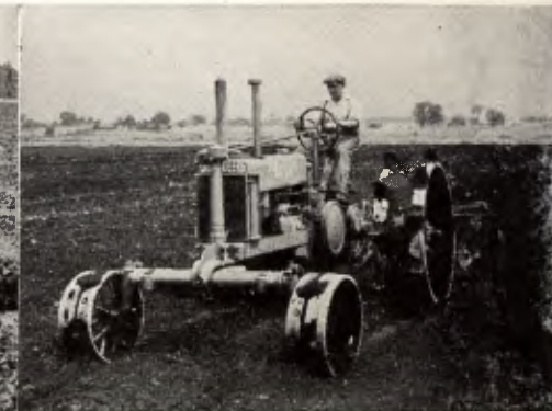
Where conditions are particularly difficult, wheels can be equipped with extension rims. The tractor stays on top of soil as soft as that shown here.
