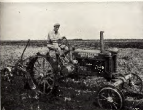
In soil so friable that it is impossible to hold a furrow wall, the Model "AW" and "BW" Tractors operate successfully. There is wide distribution of weight.
